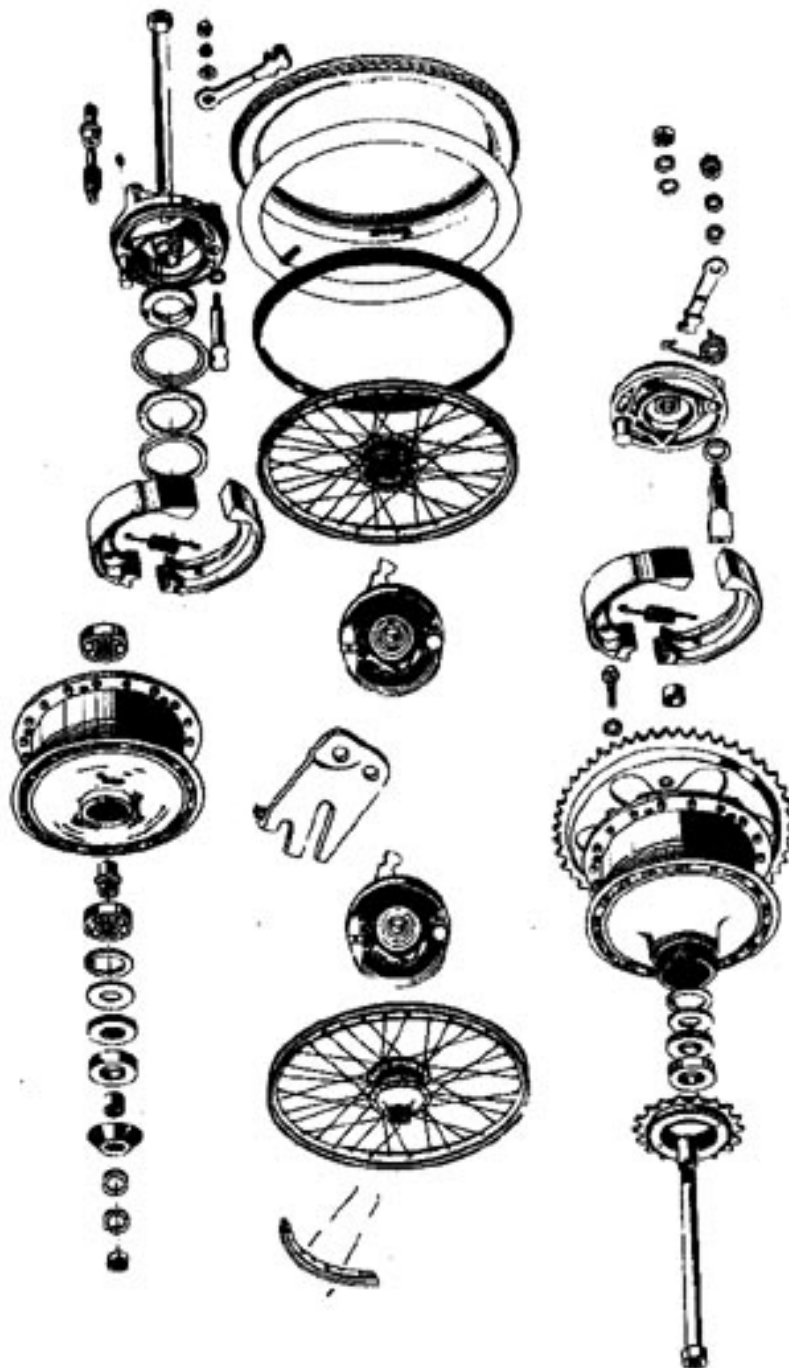
FIG. 25 Exploded view of front and rear wheel
